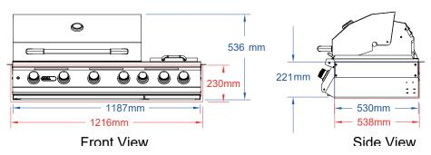
\*Red measurements shown are the recommended cut-out dimensions
