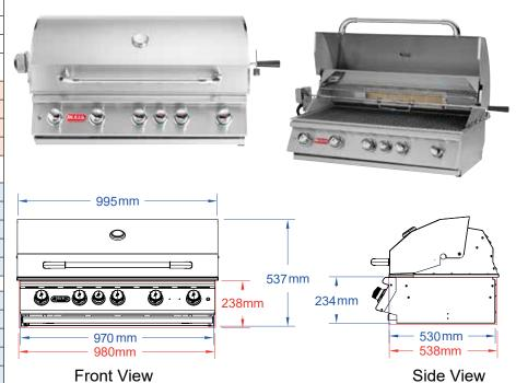
\*Red measurements shown are the recommended cut-out dimensions
