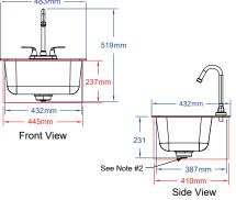
\*Red measurements shown are the recommended cut-out dimensions
