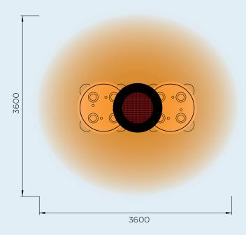
\*HEAT AREA DEPENDENT ON AMBIENT TEMPERATURE AND WIND. OPTIMUM CONDITIONS EXPERIENCED AT APPROX 15.5°C AND IN A LOW WIND COVERED ENVIRONMENT.
