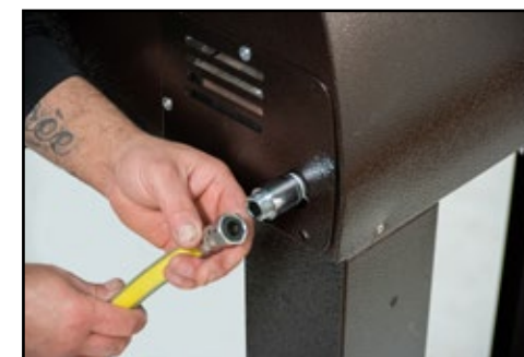
4. Screw the hose to the oven with the help of the right spanner to securely fasten it.
